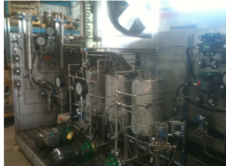
Electrodialysis Test Unit ElectroSep Test Facilities Saint Lambert, Quebec
